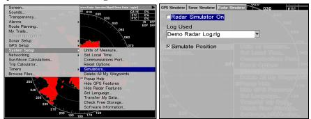
Simulators highlighted on the System Setup menu (left). Radar Simulator On selected on Radar Simulator menu (right). Notice the simulator has not been turned on, since the checkbox is unchecked.
